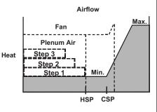
Variable Volume Fan VAV Terminal with Proportional Water Heat
