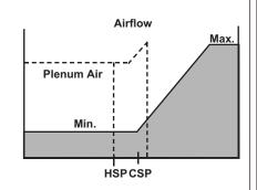
Variable Volume Fan VAV Terminal with Electric Heat
